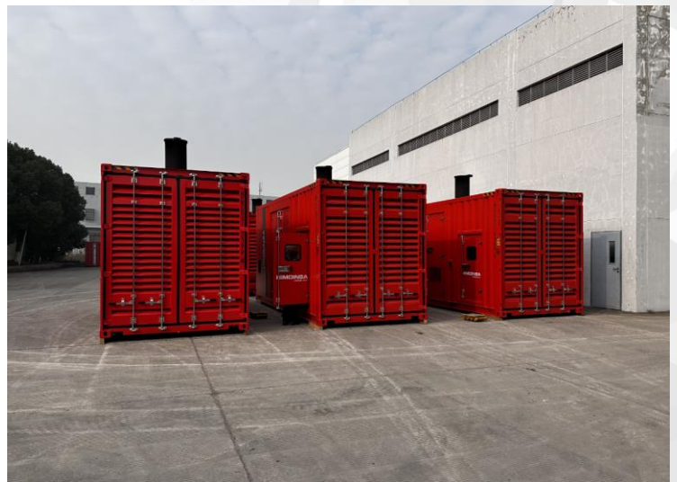
Figure 3: Portion of the burner system (left) and backup generators (right) post factory acceptance testing and pre loading in China.
