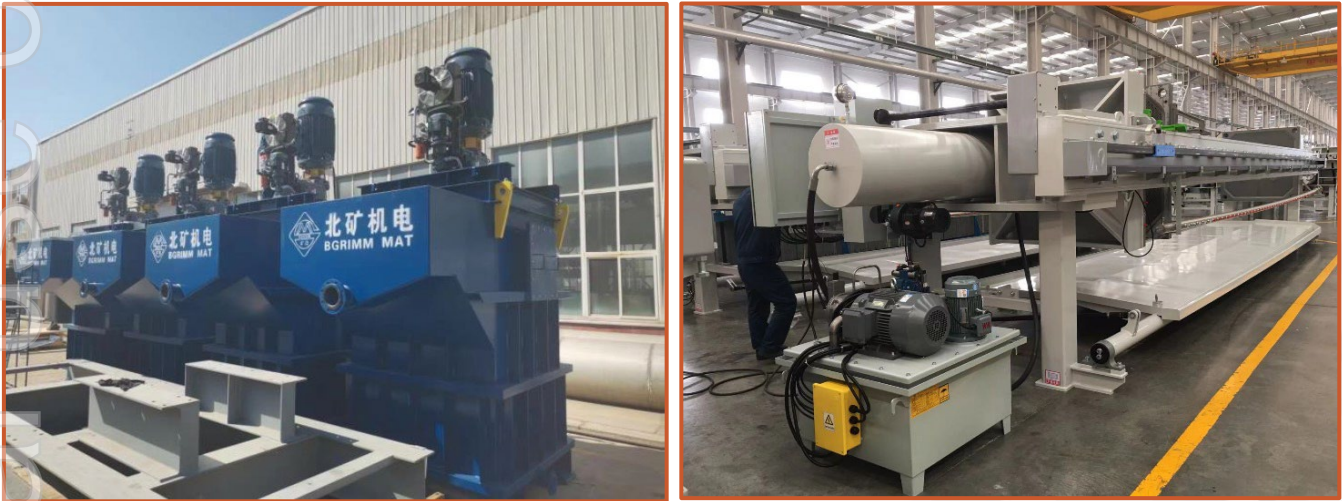
Figure 2: Factory acceptance tests of the BGRIMM attritioning mills (left) and filter press (right).
