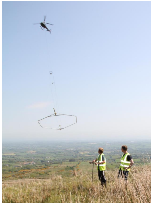
Figure 1: Heliborne SkyTEM survey over the Tyrone JV Licence with Company geologists conducting soil sampling in the foreground.
