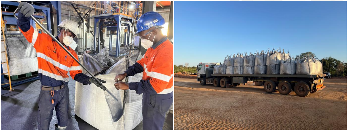
Figure 2: Sampling of bagged concentrate (left) and loading of a consignment to the port warehouse (right).
