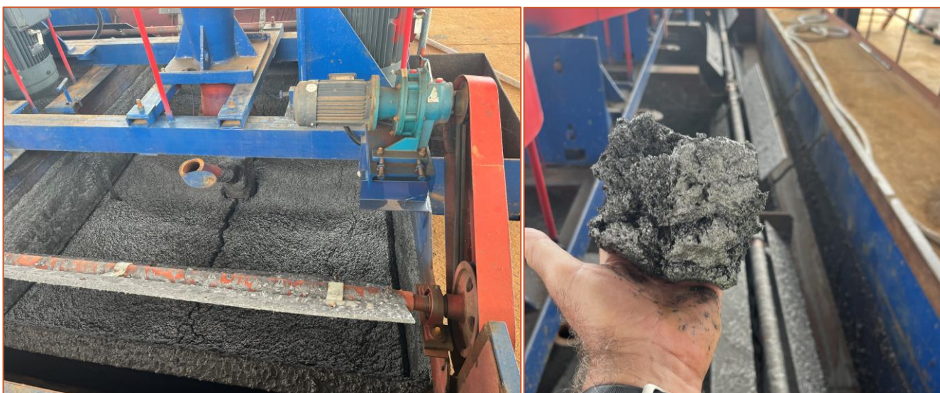
Figure 1: Lindi Jumbo graphite flotation (left) and graphite concentrate cake (right).
