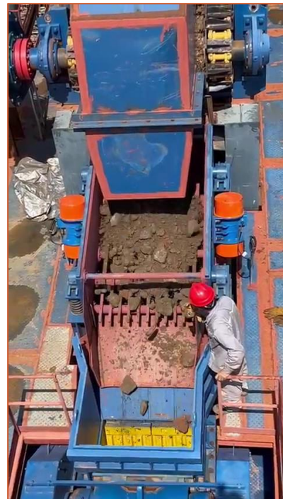
Figure 1: First feed of graphite ore to the ROM bin (left) and feed over the vibrating grizzly (right).
