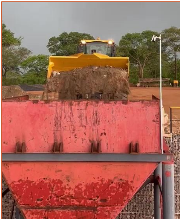
Figure 1: First feed of graphite ore to the ROM bin (left) and feed over the vibrating grizzly (right).
