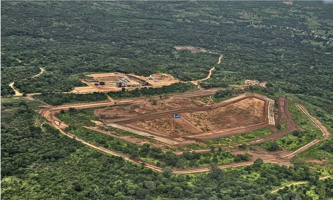
**Figure 3: Aerial photo of the Lindi Jumbo Project from the northeast taken at the beginning of April. Rockfill embankment progress at the TSF can be seen in the foreground.**
