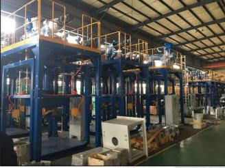
Figure 2: Manufacturing of the Rotary drier (left) and the concentrate bagging equipment (right).
