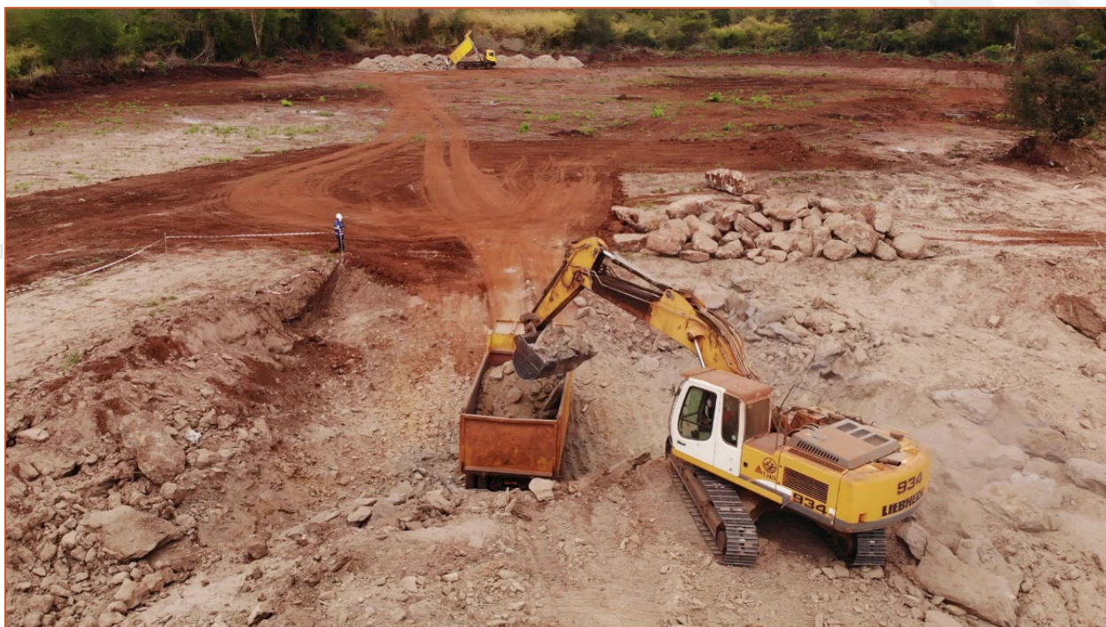
Figure 2: The box-cut being opened with the loading and hauling of the fragmented blasted material. The temporary high-grade stockpile is in the background.
