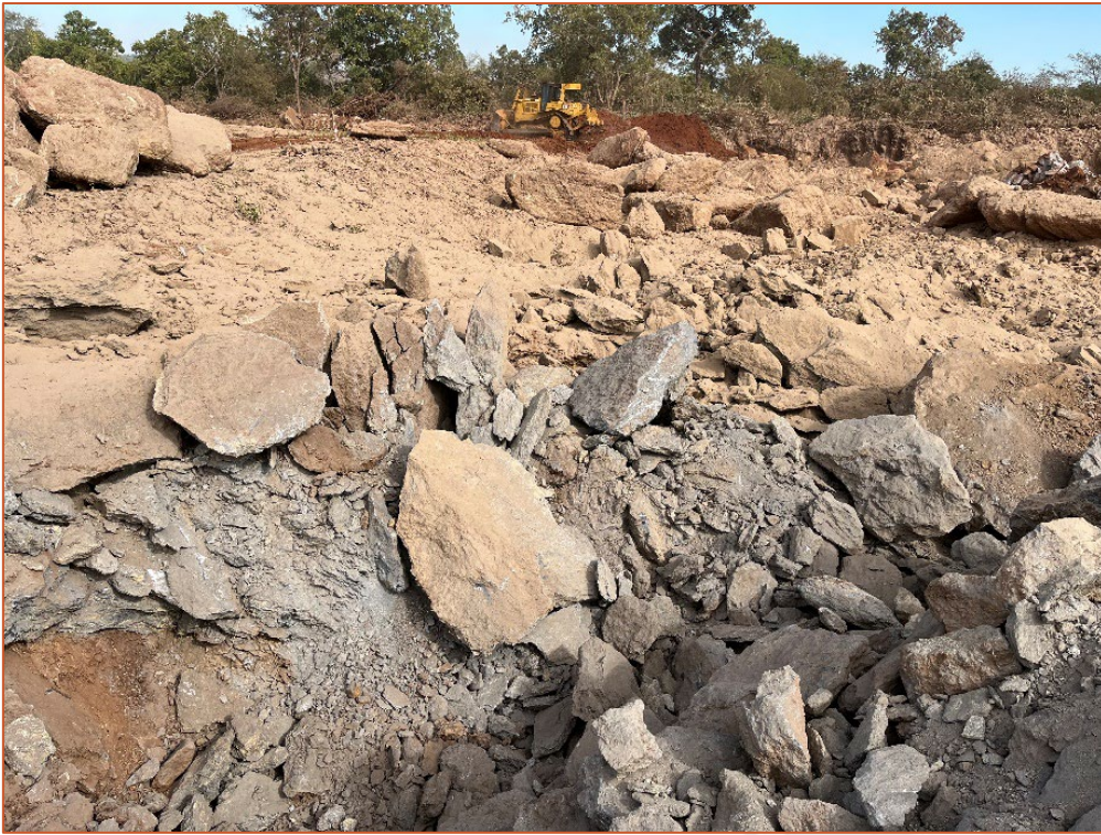
Figure 3: A visually distinct high-grade graphitic ore zone (dark grey) within the starter pit area. The grade of the exposed graphite ore is estimated to be between 30% - 40% TGC.
