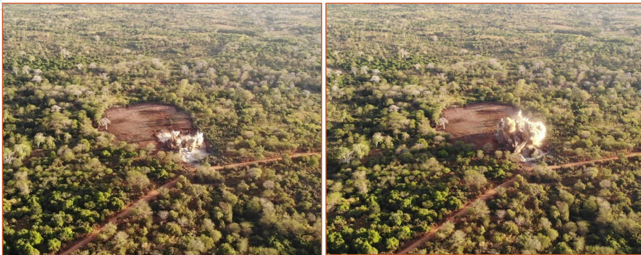
Figure 1: Blast sequence at the starter pit looking south. The main super high-grade zones are approximately 30m to 50m to the east (left) of the blast zone and strike NE-SW.
