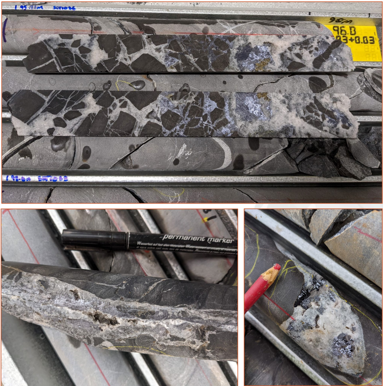
Figure 2: Selected photos of mineralisation in core. Top: galena and sphalerite within the quartz-carbonate breccia (BCRDD-002). Bottom (left) Galena stringer zones within quartz-carbonate vein (BCRDD-001) and (right) Galena vugs within quartz-carbonate vein from BCRDD-003.
