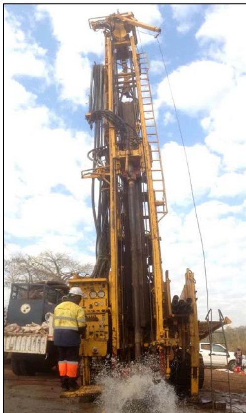
Figure 3: Water blown out of the standpipe during drilling operations.
