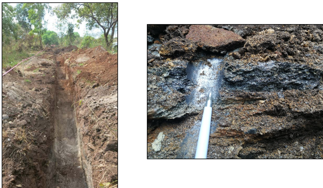
Figure 2: (Left) Trench LJTR008 with high grade zone in the immediate foreground. (Right) High-grade weathered graphite schist in trench.
