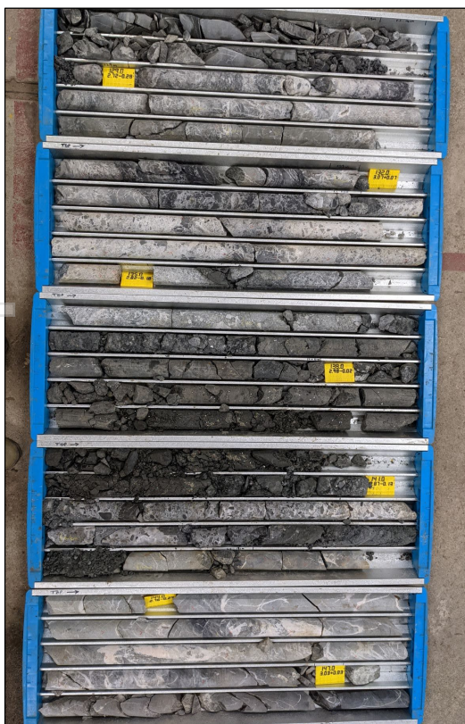
Figure 6: Left - Brecciated and altered "ore zone" in Drillhole BCRDD002 from 129m to 147m downhole. Right - galena (lead sulphide) and sphalerite (zinc sulphide) within the breccia zone.
