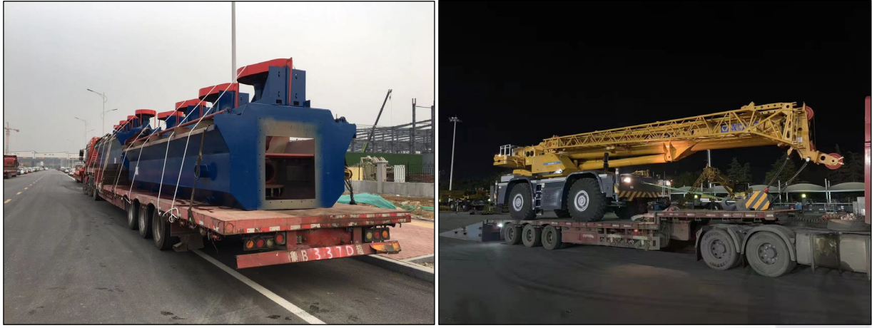
Figure 1: Large floatation cells (left) and mobile crane (right) being transported to the Port of Shanghai
