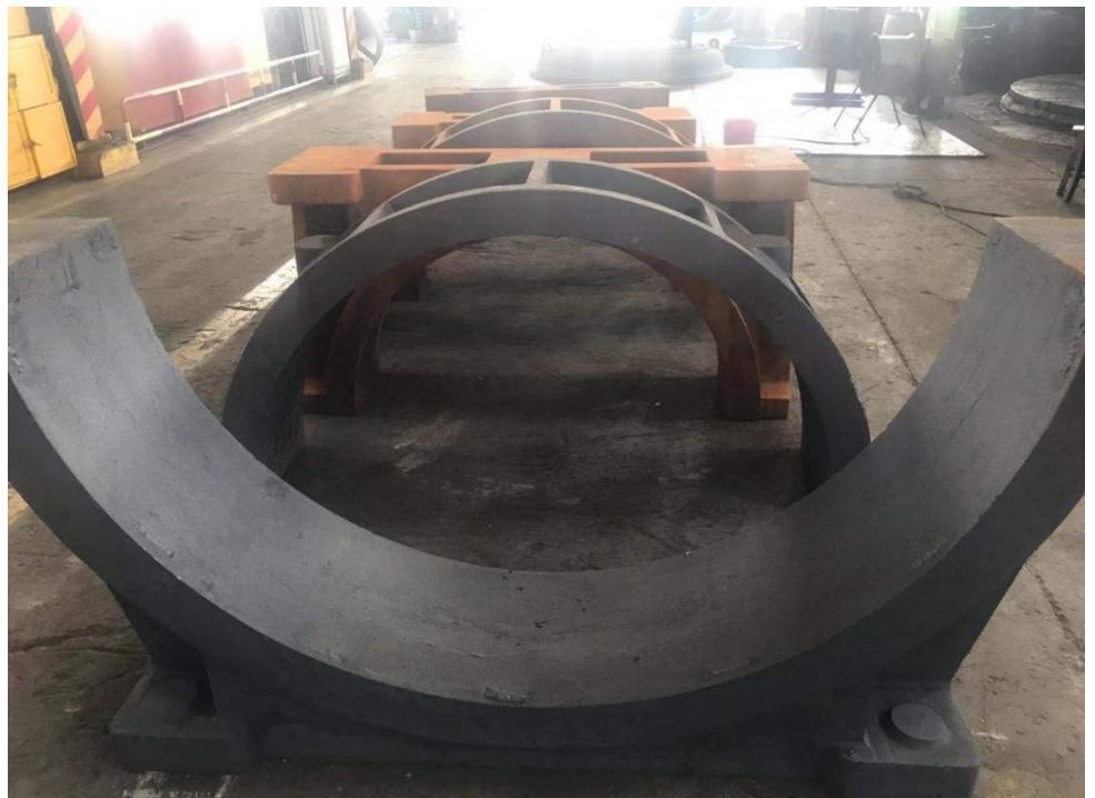
Figure 1: Photo of Lindi Jumbo mill bearing bush being readied for machining.
